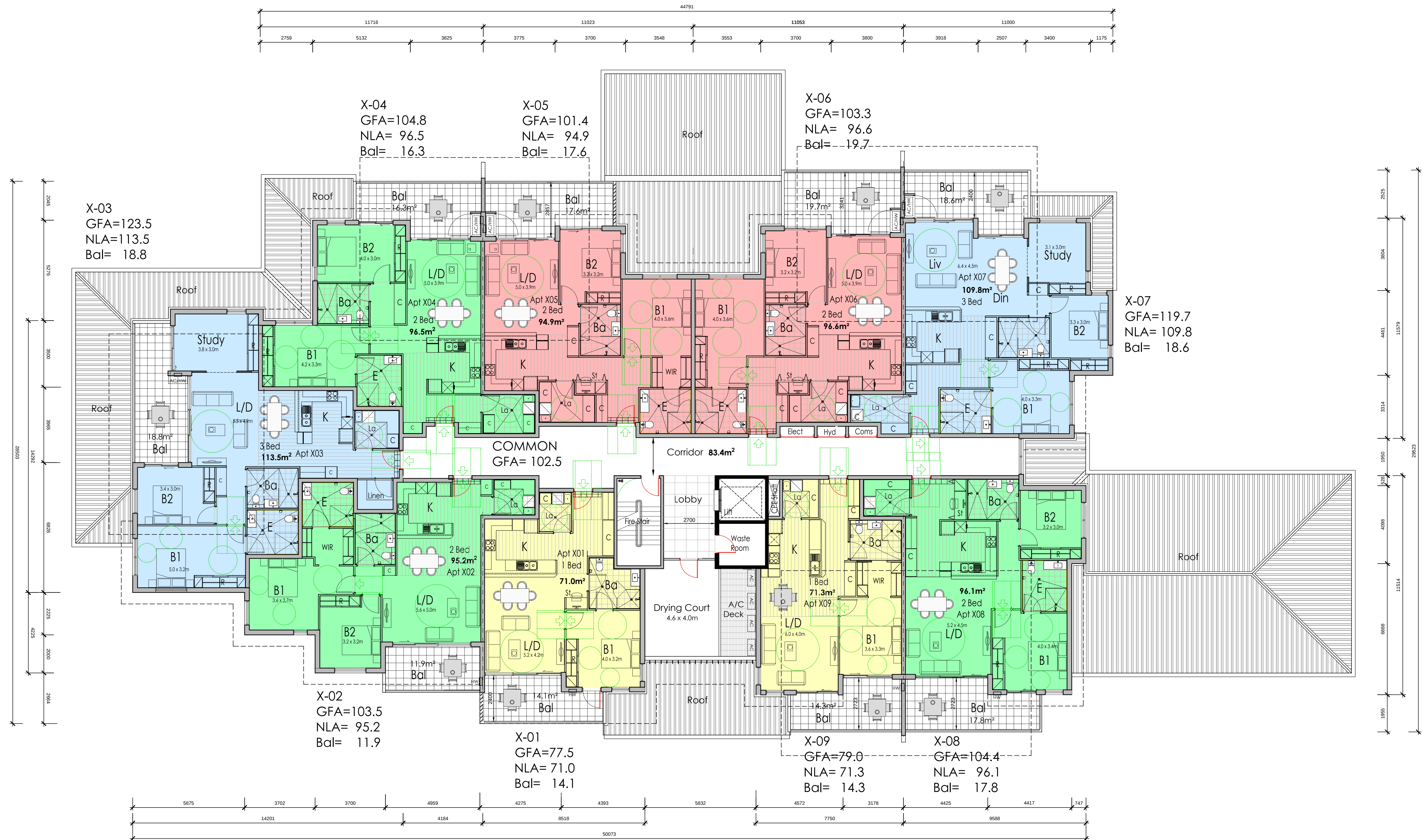
1 ILU BLOCK E TYPICAL FLOOR PLAN 1 : 100
